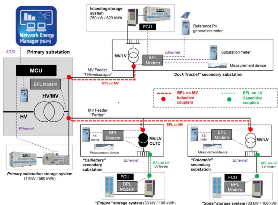
Figure 1 - Overall BPL communication architecture
