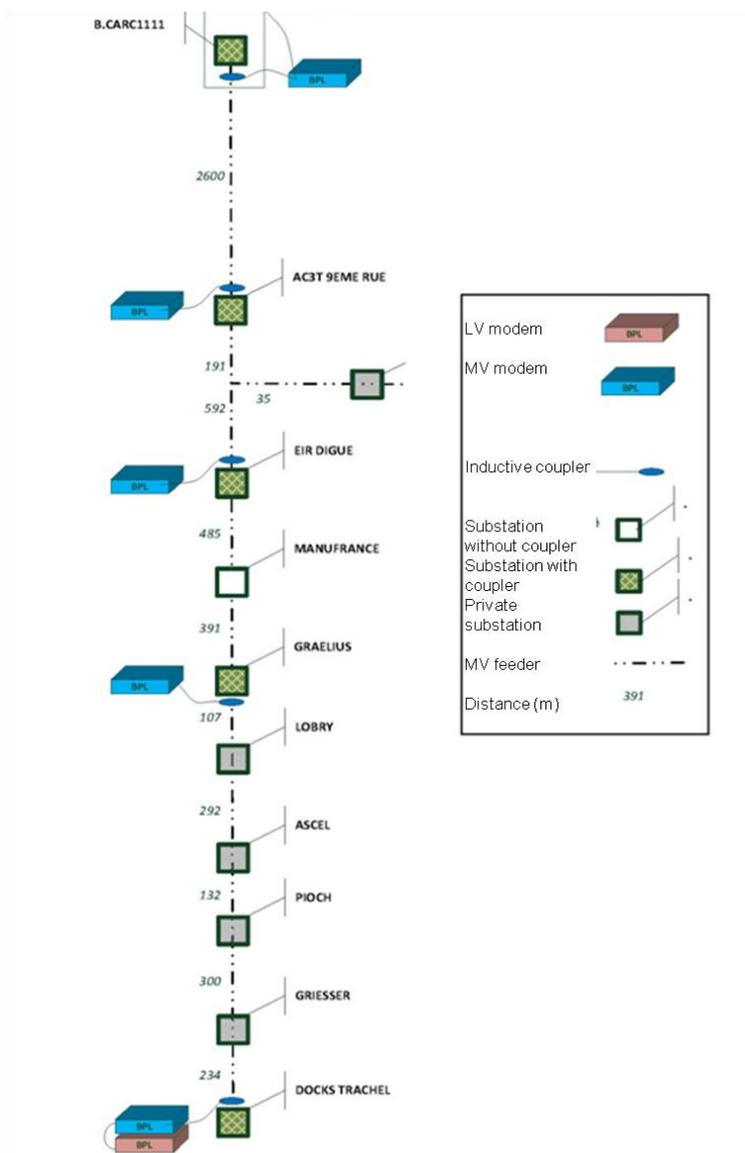
Figure 2 - BPL modem setup at the “Telemecanique” outgoing MV feeder
