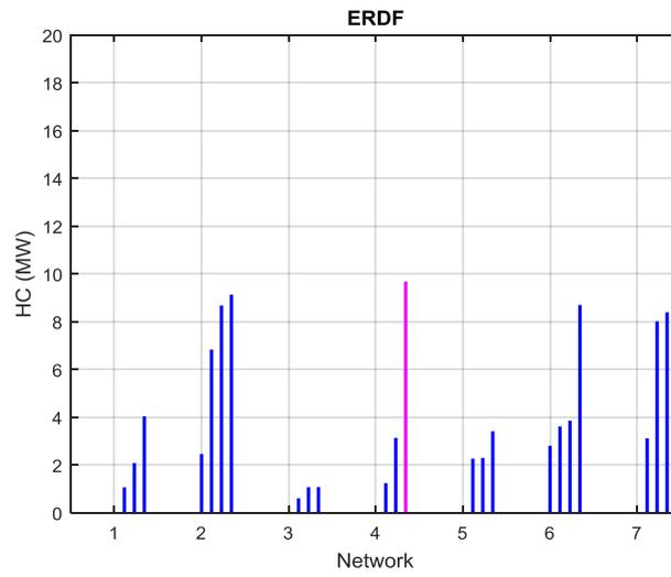
Figure 4: (Hosting capacity per feeder for the ERDF networks - example)
